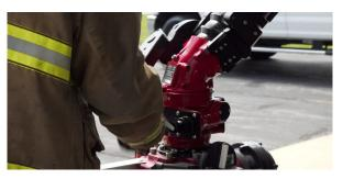
Flex provides an extensive range of motion, with 165 degrees of vertical travel (120 degrees above horizontal and 45 degrees below horizontal) and 225 degrees of horizontal travel to the left and right, totaling 450 degrees. This wide range allows firefighters to cover broad areas with precise control, ensuring optimal water placement for various firefighting scenarios, whether reaching high elevation fires or targeting low-angle areas.
